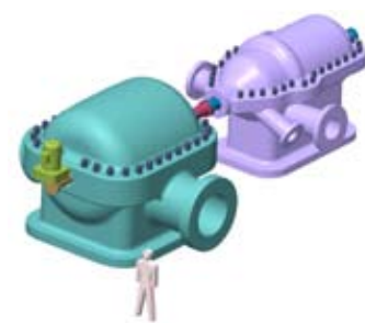
Supercritical CO 2 Cycle Turbine and Compressor
